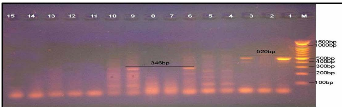
Fig 2. Ethidium bromide-stained agarose gel of multiplex PCR amplified products from extracted DNA of bla AmpC positive K.pneumoniae isolates and amplified with bla ACC and bla MOX genes primers (forward and reverse). Lane (L), DNA molecular size marker (2000-bp ladder), Lanes (1 and 3) of K.pneumoniae isolates showed positive results with bla MOX (520 bp) genes and Lanes (6 and 9) showed positive results with bla ACC (346bp) gene.
